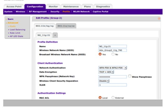
Edit Group-2 802.11a/na/ac tab for SSID configuration Keep the Profile name as a default i.e Name :NG\_11a-21 and Broadcast Wireless Network name (SSID) : Adv\_Group2\_11a\_740
