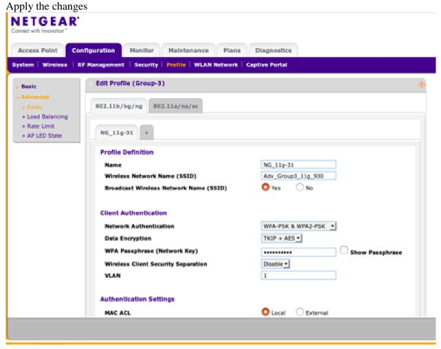
Edit Group-3 802.11a/na/ac tab for SSID configuration Keep the Profile name as a default i.e Name :NG\_11a-31 and Broadcast Wireless Network name (SSID): Adv\_Group3\_11a\_930
