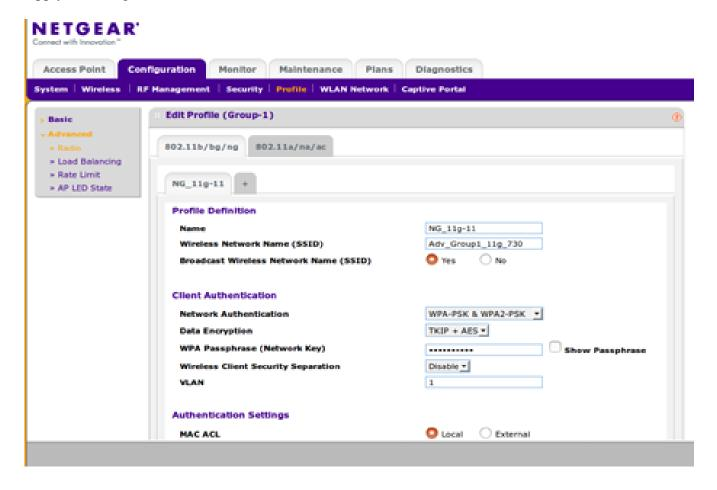
Edit Group-1 -802.11a/na/ac tab for SSID configuration Keep the Profile name as a default i.e Name :NG\_11a-11 and Broadcast Wireless Network name (SSID) : Adv\_Group1\_11a\_730
