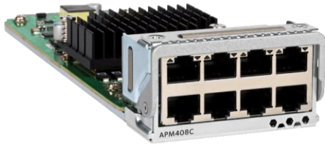
8x10GBASE-T PoE+ Port Card - 100M/1G/2.5G/5G/10G (APM408P)
