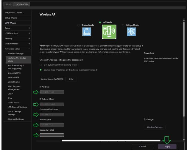
After input boxes have been filled in correctly and checked, select the APPLY button.
