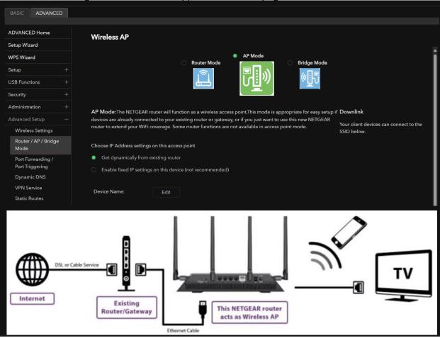
Select the **Enable fixed IP Settings on this device** radio button. This will display the **IP Address, IP Subnet Mask, Gateway IP Address, Primary and Secondary DNS** configuration input boxes:
