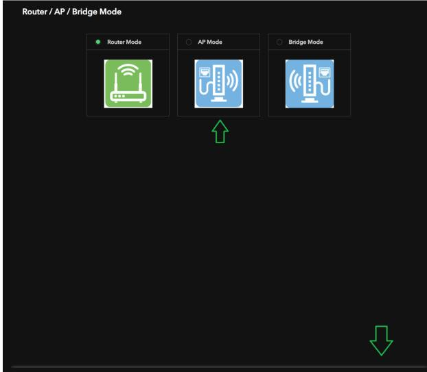
Select on the **AP Mode** tile to select this mode for the NETGEAR router.
