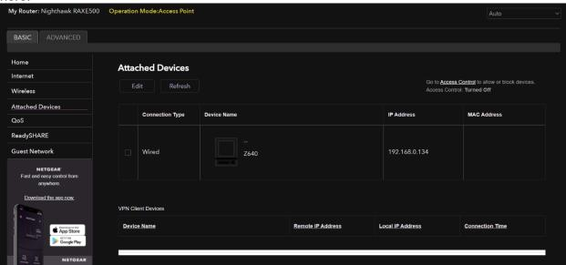
Check with all connected devices that they can connect to the NETGEAR router in AP mode. Verify they get internet services while connected.
