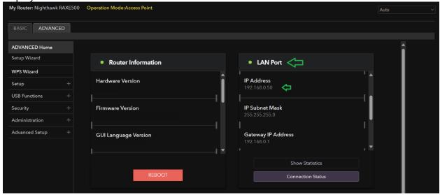
Users can now configure the wireless settings or configuration on the NETGEAR router as desired. Navigate to the **Basic Tab/Wireless Settings** web page to make changes here.
