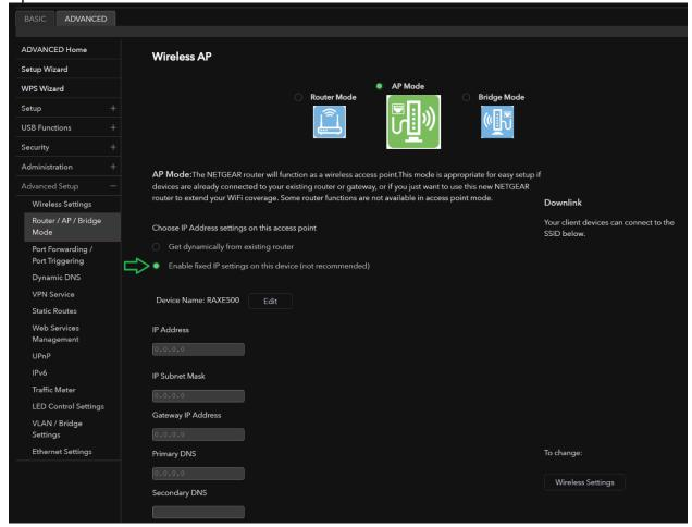
Configure the **IP Address** box for a static IP address number that is outside of the host routers DHCP IP Address pool range. Recommend setting the default DHCP IP address pool range to the following after applying and a factory reset: 192.168.#.100 to 192.168.#.200.
