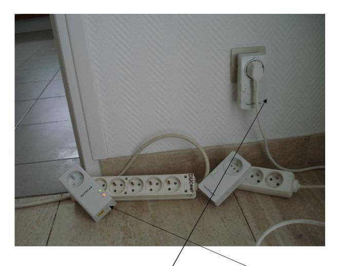
Depressing the Security button for more than two seconds on the PLP 1000 unit. The PLP1000 "Power" LED is flashing.
