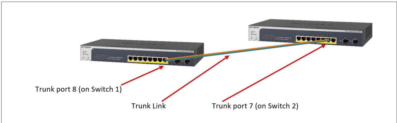
**VLAN tagging (on trunk port):** Tagging VLAN 2 on a trunk port ensures VLAN 2 ID is inserted into all data packets forwarded from VLAN 2 before they exit the switchport. This helps identify the data packets as belonging to VLAN 2 on the other switch.
