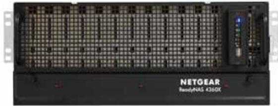
The RR4360S is a 4U 60-bay high-density storage system which supports SATA/SAS/SSD hard drives. With a high-performance Intel Xeon processor and 16 GB ECC memory, the software level provides comprehensive data protection with 5 levels of data protection. Mainstream RAID levels such as RAID 5/6/10/6/5 are supported. High-density storage meets the stringent requirements of space/capacity.
