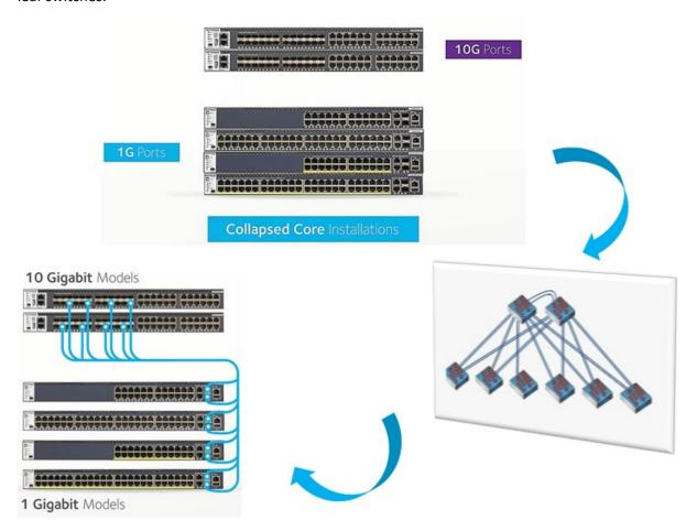
This six-switch spine and leaf design would be the typical topology for an SMB datacenter or branch office installation. The six M4300 switches are stacked together in a spine and leaf topology using two of this 10Gbps uplink ports 27,28 (M4300-28G) and 51,52 (M4300-52G) on each leaf switch and four 10Gbps ports on each of the M4300-24X-24F switches as the spine. The stacking and uplink connection would be configured at follows.
