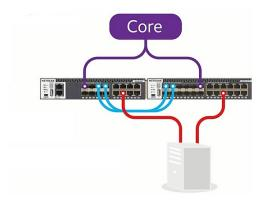
The two-switch M4300's would be the recommended topology for a small and mid-sized business. The two switches are connected horizontally with ports 1/0/5 and 1/0/7 on switch 1 and 2/0/1 and 2/0/3 on switch 2 as the 10Gbps stacking ports. Ports 1/0/1 and 2/0/11 are used as a dual-homed uplink to the core switch. The rest of the available switch ports on both switches can be used with servers running LACP and active-standby configuration on the server side NICs.
