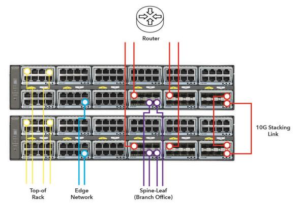
The pair of M4300-96x's are stacked on (8) 10G ports (1/12/5-1/12/8 on switch 1 and 2/12/5-2/12/8 on switch 2) for a total stacking bandwidth of 20G bi-directional. The rest of the ports on both redundant core switches are used for downlink connectivity when using top-of-rack, edge networking, and spine and leaf networking.
