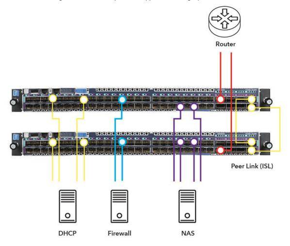
The two-switch M4500 top-of-rack solution is a recommended topology for a small and mid-sized business. The M4500 brings huge benefits for top-of-rack architectures. In the above topology, the two M4500-48XF8C's are connected between each other with ports 0/55 and 0/56. The ports are connected with LACP and has MLAG configured between the both. MLAG protocol introduces the layer 2 high availability redundancy that a top-of-rack environment would require when a failure occurs with one of
