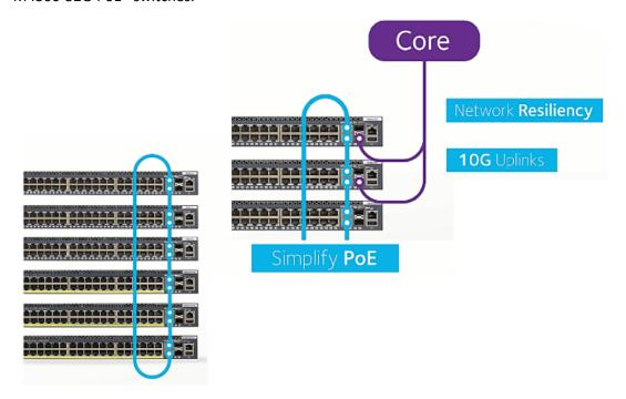
This six switch M4300 design would be the typical edge switch topology for an SMB infrastructure. The six M4300 switches are stacked together in a ring topology using two of the 10Gbps uplink ports (49 and 50) on each switch. The stacking and uplink connection would be configured at follows.
