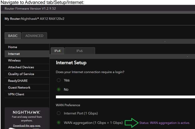
Under WAN Preference for WAN aggregation (1 Gbps + 1 Gbps) the status will display WAN aggregation is active. This means the Link Aggregation connection between the cable modem and router is good and working.
