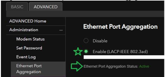
Ethernet Port Aggregation Status should display Active in GREEN. This means the Link Aggregation connection between the cable modem and router is good and working.
